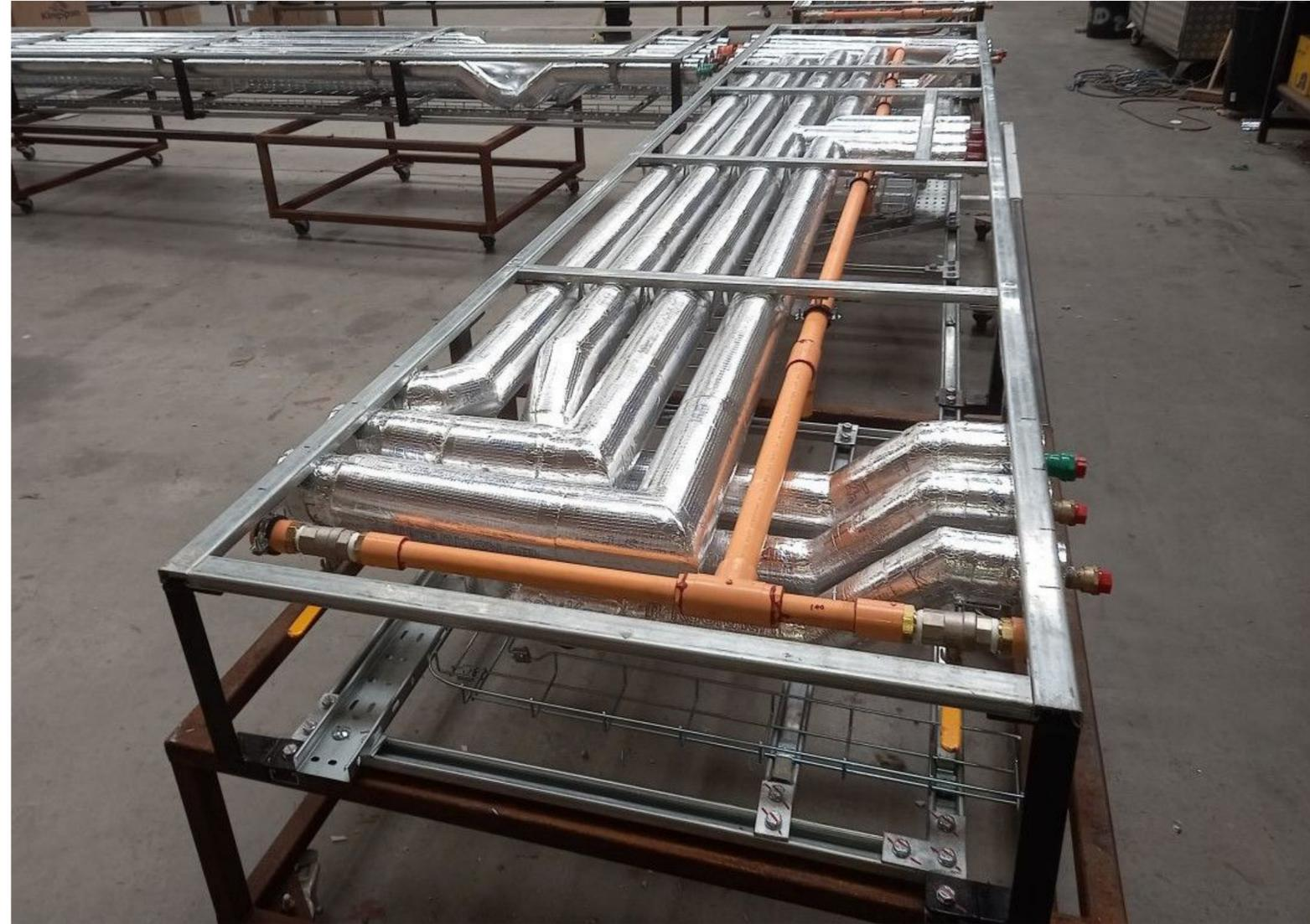
Pre-fabricated modular MEP based on 3D
